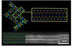
An experimental image and a theoretical model of nanowire Ta-Pd-Se with a diameter 2.1 nm. The foundation of the structure a separate nanowire Ta2Pd3Se8 as highlighted in a frame.
