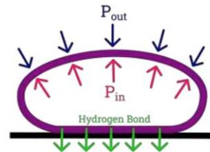
Fig.4. Various Force inside & outside the bubble
