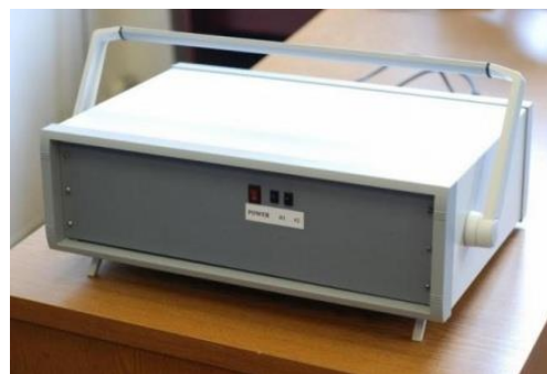
IR spectro-radiometer to identify greenhouse gases and measure their distribution.
