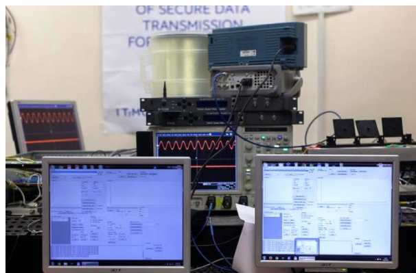
Experimental device of quantum cryptography system.
